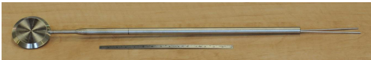
Figure 1 - A disk assembly (prior to support tube bending) showing the disk on the left, support tubing (center), and pressure tap tubes extending to the right. All materials are 304 stainless steel. A 150 mm straightedge is shown for scale.
