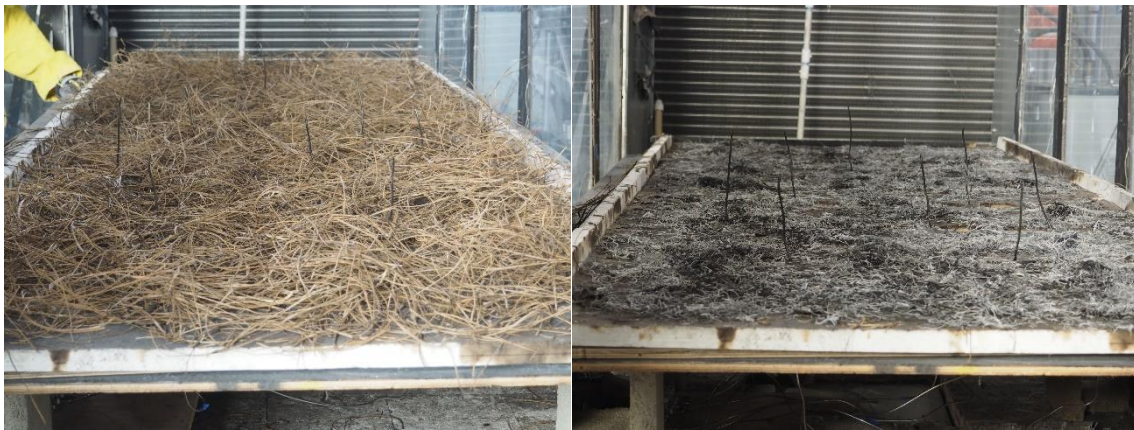
Figure 4 - Canister gas-sampling system with manifold (top) used to sample pyrolysis and flaming combustion gases from longleaf pine needle fuel beds through stainless steel tubes (bottom).
