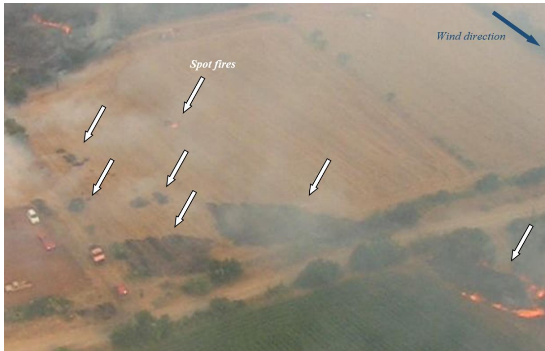
Figure 4a - An along-wind pattern of landing embers, on grass, downwind from a surface head fire
