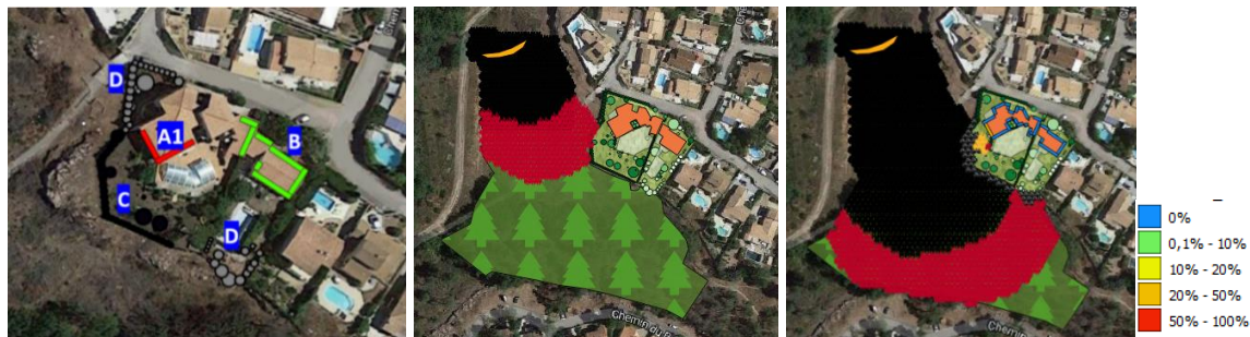
Figure 5 - Rognac fire: comparison between the observed (left) and predicted damages after 300 s (middle) and 600 s (right) of fire. For the two latter, the red areas correspond to the burning areas, the black ones to the areas burnt due to crowning, and the grey ones to the areas burnt from surface fire. Contour legend gives the percentages of panels damaged by fire on each building facade.
