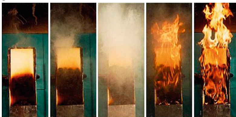
Figure 3 - Series of photographs of a combustion experiment illustrating the transition to flaming in a smouldering foam slab 40 cm high under external forced flow (Photo by group of Prof. Carlos Fernandez-Pello, University of California at Berkeley). After 1 h of smouldering only half the sample has burned (Photo 1, far left). When the rapid transition to flaming takes place (Photos 2 and 3), the whole sample is engulfed in flames in just a few seconds (Photos 4 and 5, far right)
