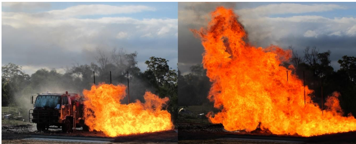
Figure 4. CFA Medium tanker on the flame front simulator during the 25,000kW/m 2 Mogo, NSW, experiment
