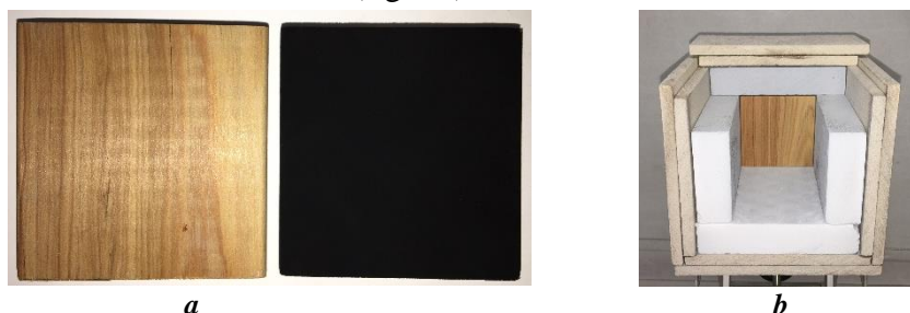
Figure 2 - a) Original (left) and blackened (right) sample; b) sample holder to block convection cooling
