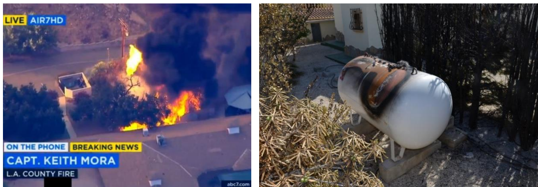
Figure 2 - Left: Calabassas fire (California, 2016). A propane jet fire can be observed at the centre of the image. Flames from ornamental fuels are close to the tank. LPG infrastructure was inside a kindergarten facility. Right: Domestic LPG tank in Benitatxell (Spain, 2016) damaged by the jet fire. The tank was surrounded by an ornamental hedgerow that ignited by spotting.
