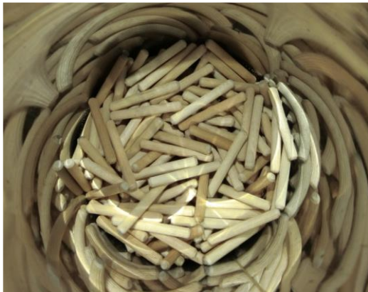
Figure 7 Fuel batch loaded in firebrand generator
