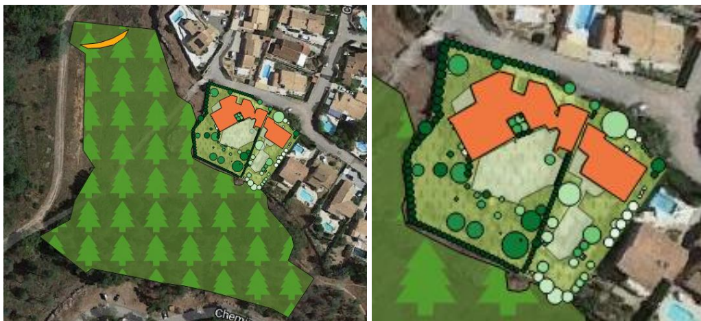
Figure 4 - Rognac fire: visualization of the initial fire front position and the different polygons used to model the natural and ornamental vegetation (in green), non-combustible materials (in grey; swimming-pool, concrete areas, etc.), and combustible material (in orange).
