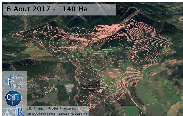
Figure 3 - Rapid-Response simulation, without firefighting actions. Fire as pink 20 minutes isolines, 7 hours total duration.
