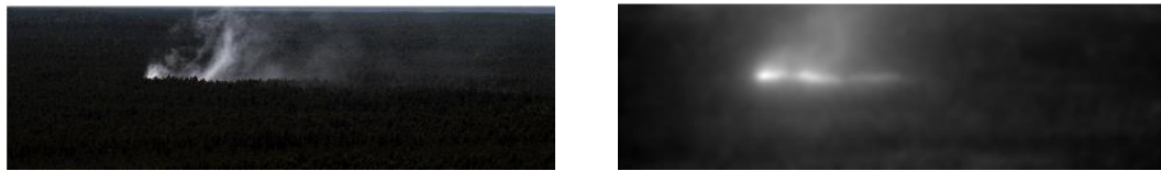
Figure 2 - Real smoke image (left), resulted energy image (right)
