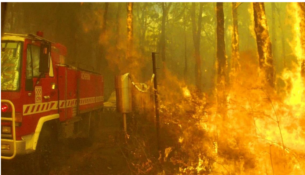
Figure 2. Brucknell experimental burn impacting the CFA medium tanker, CAFS and Gel ultra-light tankers
