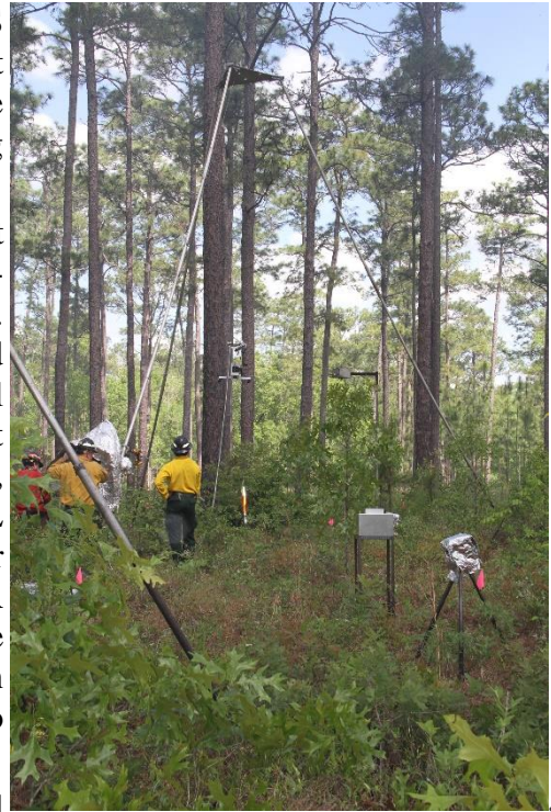
Figure 2 - In-situ infrared tripod system, FBP and video sensors.
