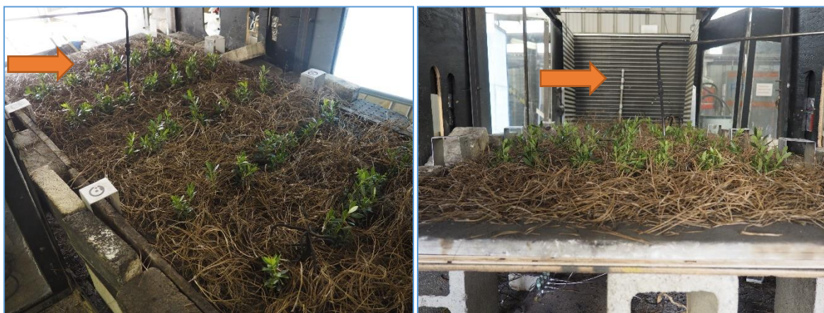
Figure 3 - Fuel bed composed of longleaf pine needles and Lyonia lucida plants. Sample probe to collect pyrolysis gases for the Bruker Tensor 37 is indicated by the arrow.
