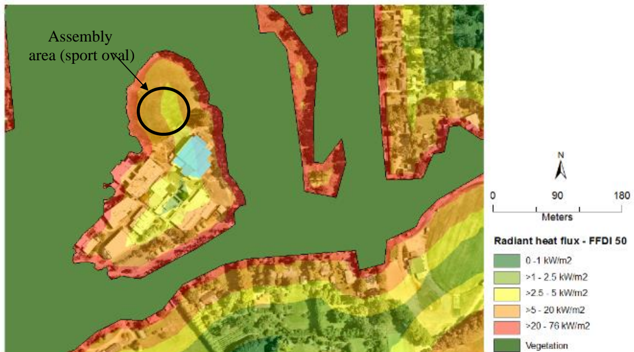
Figure 4 - Radiant heat flux exposure for FFDI 50.
