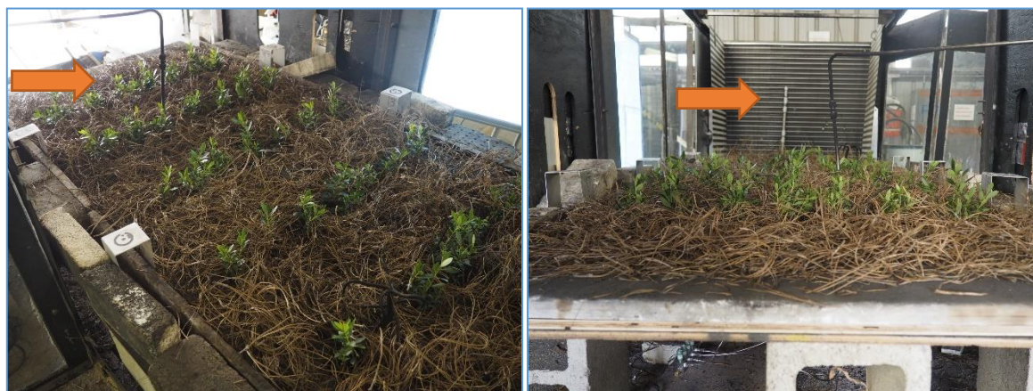
Figure 4 - Fuel bed composed of longleaf pine needles and Lyonia lucida plants. Sample probe to collect pyrolysis gases for the Bruker Tensor 37 is indicated by the arrow.
