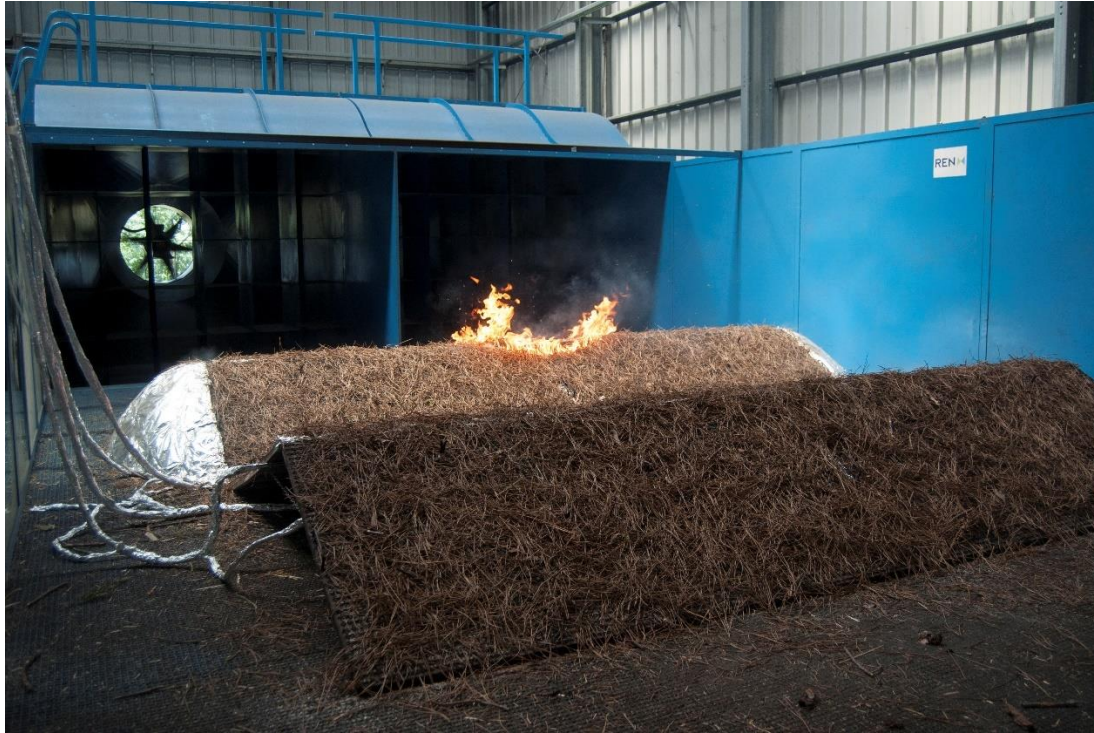
Figure 2 - Image showing the hill models placed in the wind combustion tunnel during one of the experiments, also attached the rounded ends to the left and right sides of the first hill is apparent
