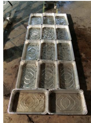
Figure 8 - Water pan arrangement for firebrand collection.
