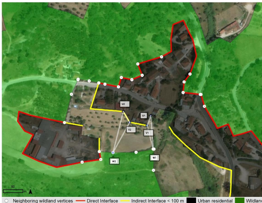
Figure 2 - WUI delineation method: the red [yellow] edges of the two urban polygons delineate the direct [indirect] WUI. Vertices U1 , V1 and W1 are nearly aligned within the 5% tolerance ( \text{dist}(U1,V1) + \text{dist}(V1,W1) < 1.05 * \text{dist}(U1,W1) ), and therefore urban vertex U1 is protected from Wildland vertex W1 by urban vertex V1 . On the contrary, urban vertex U2 is exposed to the Wildland vertex W2 , since it is not protected by urban vertex V2 ( \text{dist}(U2,V2) + \text{dist}(V2,W2) \geq 1.05 * \text{dist}(U2,W2) ).
