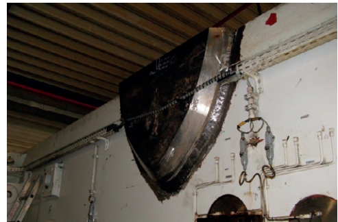
Fig. 1. Repaired fatigue breakage at a press
