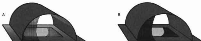
Figure 2. The two types of experimental "plexiglass" cages used to estimate Enteromorpha spp. growth: A) surrounded by 4 mm mesh size net to allow grazers entrance; B) surrounded by 0.5 mm mesh size net to prevent grazers entrance
