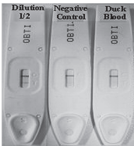
Figure 1a - Hexagon OBTI immunochromatographic test (Dilution 1/2 of human blood, Negative control and Duck blood - non human blood control).
